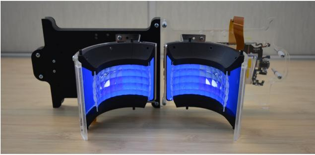
**Figure 3: Dynamic ThinVR prototype with Galaxy S9 phone displays and electronics. Displays were set to blue background to make the lenslets easy to see.**
